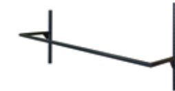
216630 - U Bar. U Bar measures 48" long on center and is 12" deep. Attaches to outriggers.
